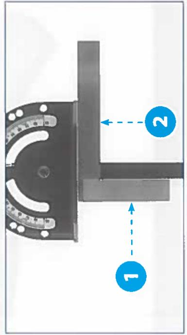
Place a square up and against the miter bar (1), next, slide it up against the face of the miter gauge (2). Set the face of the miter gauge so that it is 90 degrees to the miter bar.
