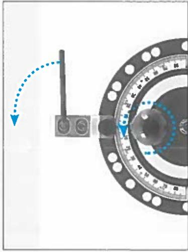
Using a hex key wrench, loosen the two set screws on the index tab of the Miter Gauge. Next, loosen the post knob handle by rotating it counter clockwise
